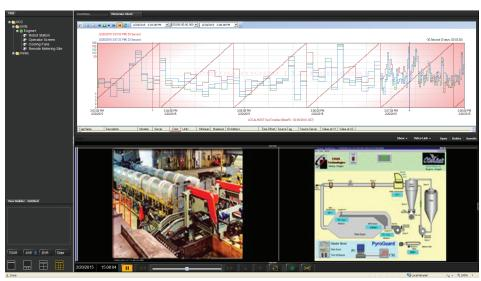
Playback of recorded operator screens synchronized with video from cameras brings a new dimension to overall process monitoring.
