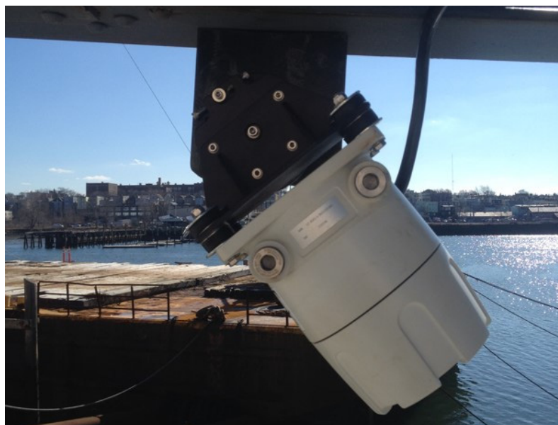
IVC's CZ-3041-2 shown mounted to a crane used to unload salt from ships at Eastern Salt's Chelsea, MA terminal.
