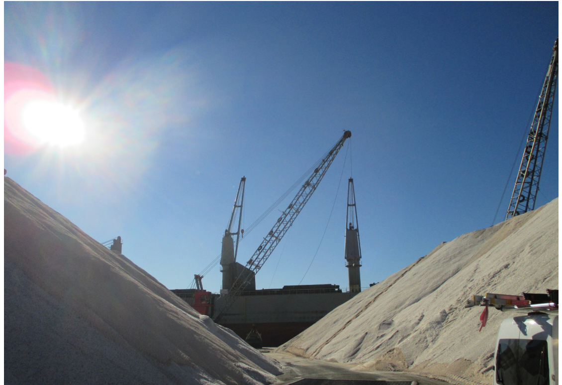
Pictured above are some of the cranes used to unload salt that's mined around the world and transported via massive cargo ships to Eastern Salt's facility in Chelsea, MA. Each crane is outfitted with an IVC CZ-3041-2 camera system. Cameras are connected to a monitor and control pad in the operator cab to give operators a better view of what is happening in the ship's cargo hold.
