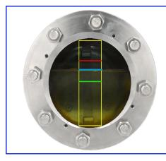
In the sight glass, the yellow rectangle highlights the area of interest. The blue horizontal line indicates the current liquid level, and the red and green lines indicate the high and low thresholds, respectively. If the liquid level crosses one of the thresholds, an alarm is generated and communicated via the Modbus or MQTT.
