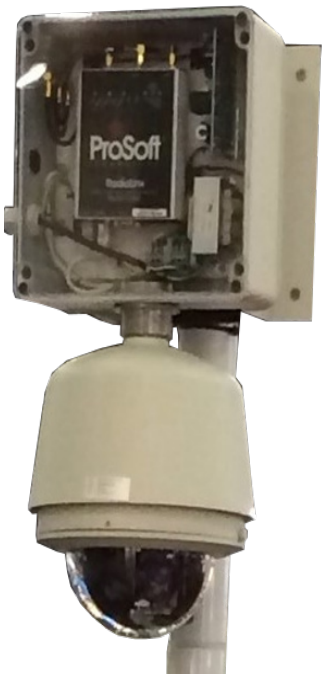
An IVC wireless PTZ camera with an integrated ProSoft Technology radio.
