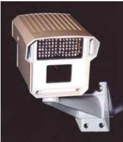
Infrared sensitive cameras with built-in infrared illuminators emitting invisible light are used to monitor the 100-foot long hallways.
