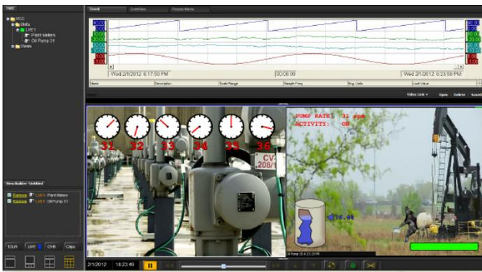
Comprehensive industrial video solutions, like those from IVC, should include video management software that integrates video with your SCADA system, turning video cameras into additional process sensors.
